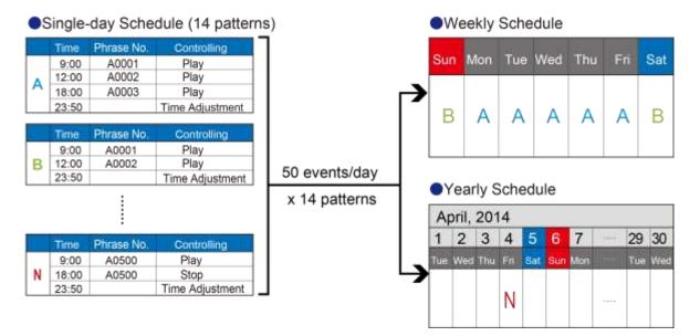
The programmable timer can be used to set the following operations (events) to occur at any specified time.
