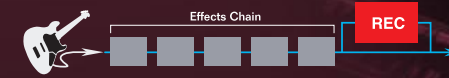
Phrase Loop placed after the effects chain: You can record the loop while switching effects on and off, making it possible to create a loop with any number of interesting FX variations.
