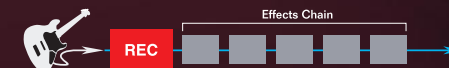
Phrase Loop placed before the effects chain: This makes it possible to record the raw performance and add or change effects after the fact.
