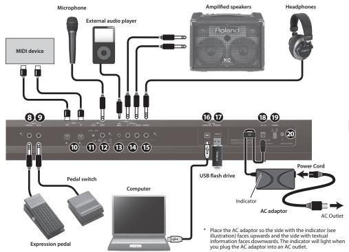
To prevent malfunction and equipment failure, always turn down the volume, and turn off all the units before making any connections.
