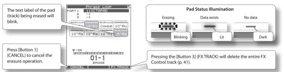
By holding down the [ERASE] button and striking a pad, you can selectively erase an unwanted portion of a track. Hit the pad at the beginning of the section you want to erase, and hit it once again at the end of the section.
