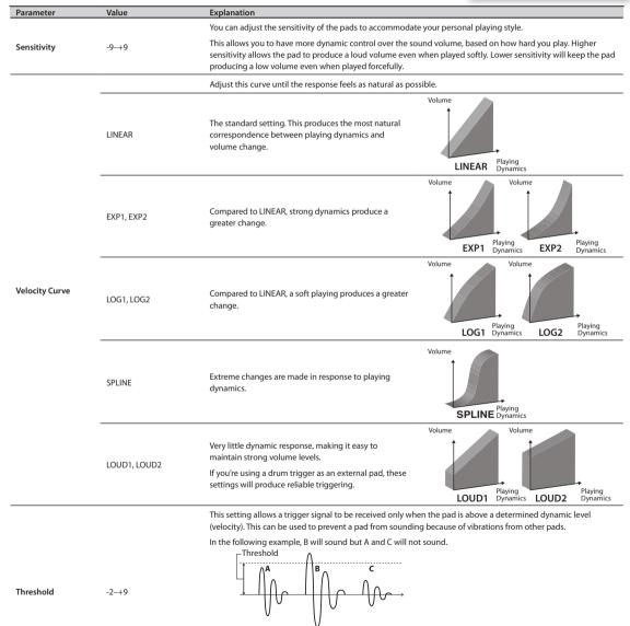
When set to a higher value, no sound is produced when the pad is struck lightly. Gradually raise the "Threshold" value while striking the pad.
